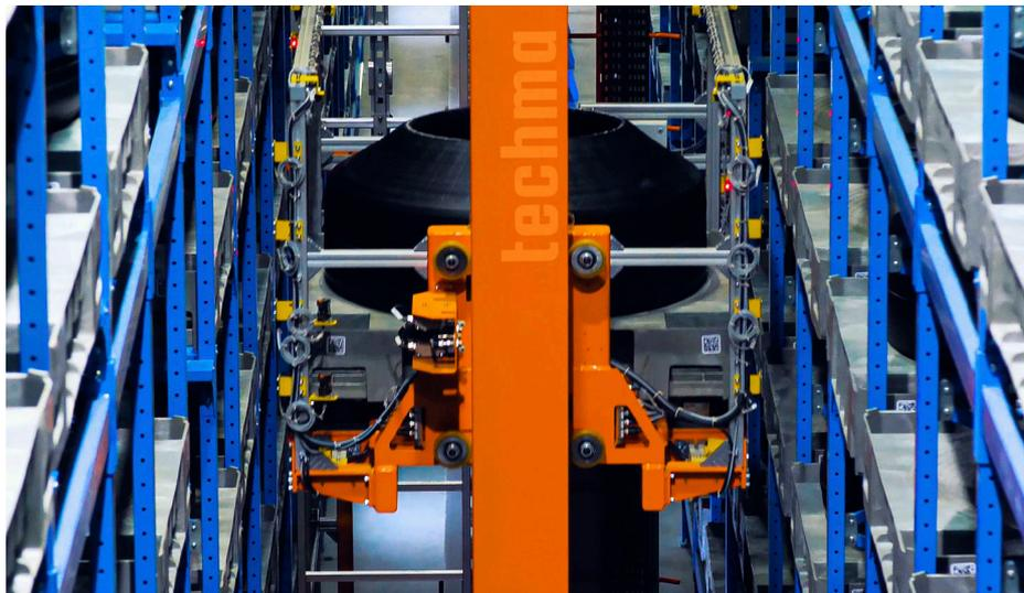
at the warehouse's exit. Tires are transferred from storage pallets to the technological oven trolleys. Additionally, the unloading system collaborates with an automated queue and trolley shifting system.
