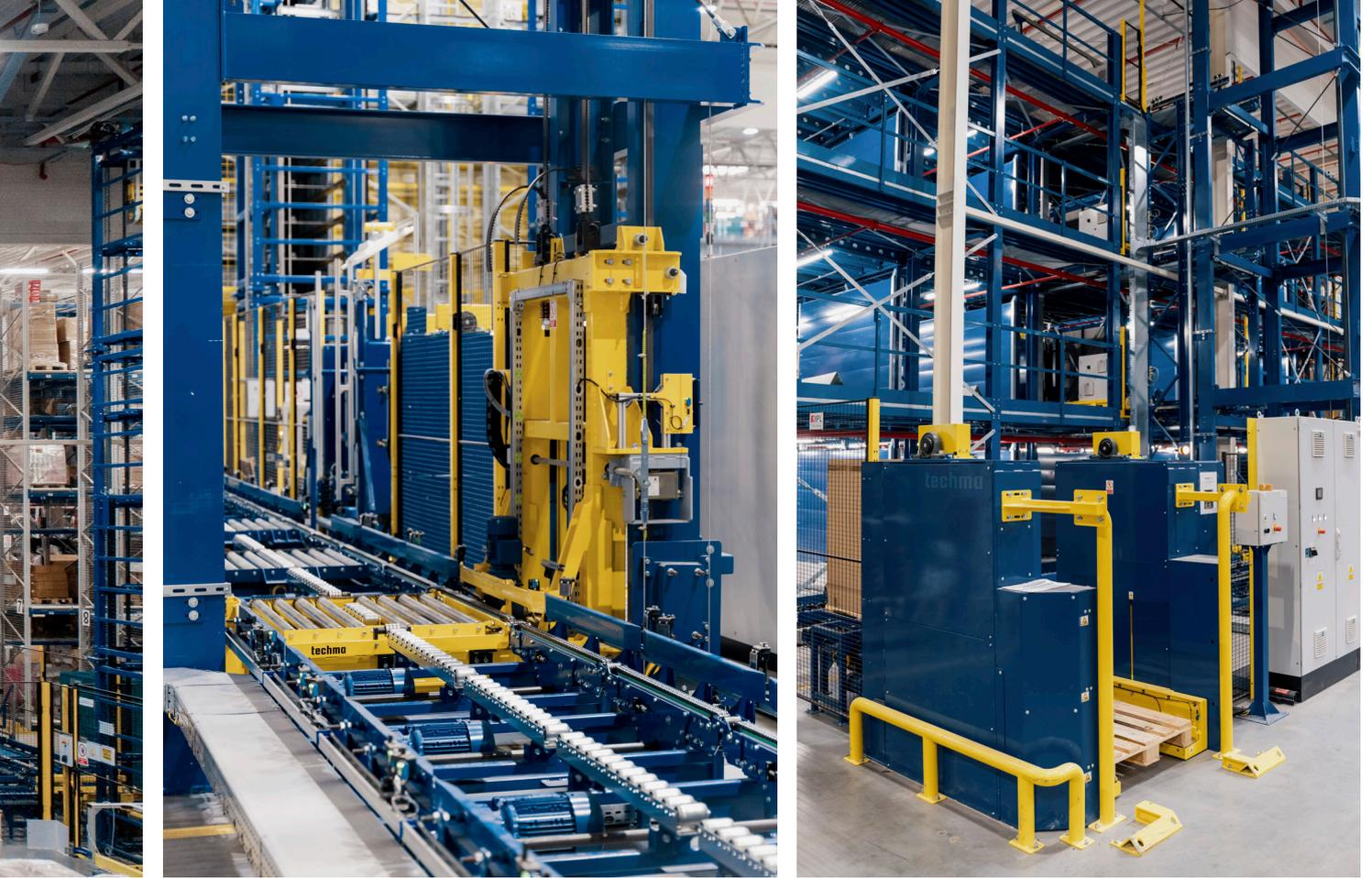
To ensure the smooth operation of the system, empty boxes are returned to the warehouse, thus completing the cycle. **The warehouse transport system is fully automated.** This means that the operator places the box on the conveyor, and it reaches the designated inspection station without the need for intervention from other personnel.
